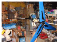
Figure 1. Behind the scenes photo of a windmill. Wind flows over the airfoil shaped blades causing lift, like the effect on airplane wings, causing them to turn. The rotation of the blades turns the drive shaft that is connected to the generator which receives energy from the shaft to produce electricity.
